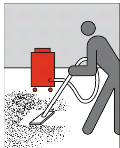
Figure 9: Dusts removed by aspiration Source: Suva
