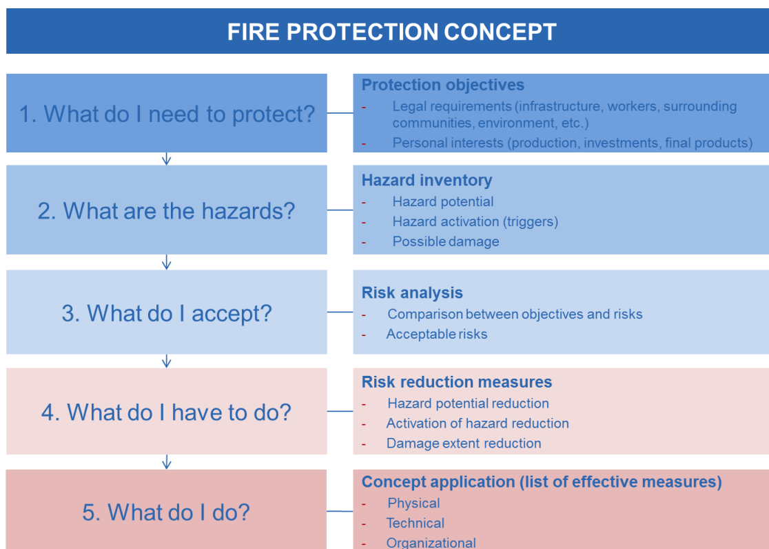
Figure 3-19: Fire protection concept [72]
