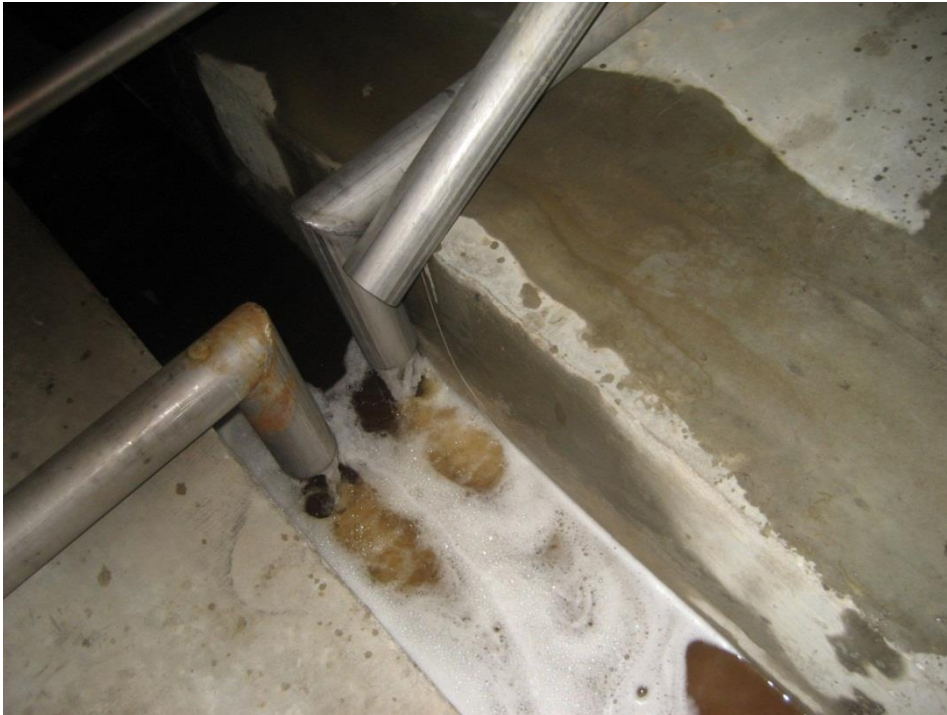
Figure 3-10: Chemical loss by uncontrolled liquor pick-up [22]
