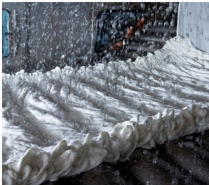
Figure 3-3: Prewash and relaxing of viscose knitwear [23]
