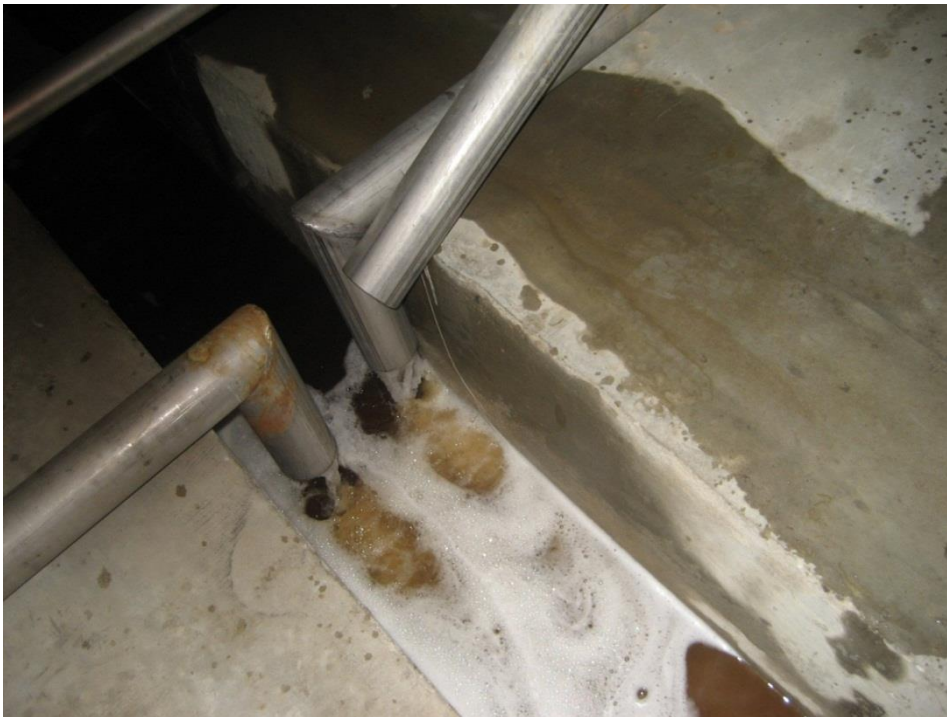
Figure 3-10: Chemical loss by uncontrolled liquor pick-up [22]
